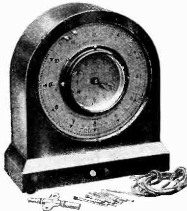
The Axuel programme selector provides a means of automatically switching on and off any number of items during the day.
